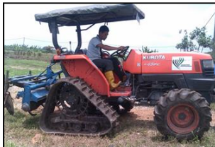
Tractors with large tracks to distribute weight over soft soil
