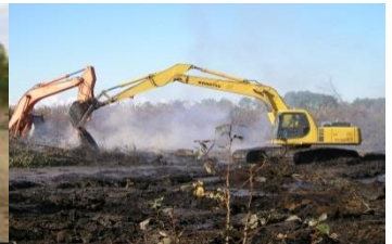
Excavators to mix water into burning peat to extinguish it
