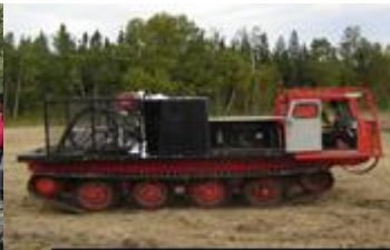
Specialised carriers with wide tracks to move crew and other supplies in and out of peatland
